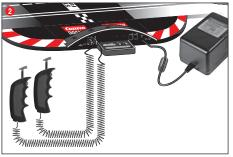
Connect the transformer plug with the Control Cont.
