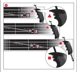
1 Make sure that the car's guide keel is located inside the track slot and that the double sliding contact is in contact with the current carrying track.
