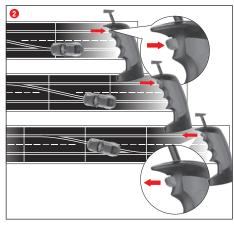
Make sure that the car's guide keel is located inside the track slot and that the double sliding contact is in contact with the current carrying track.
