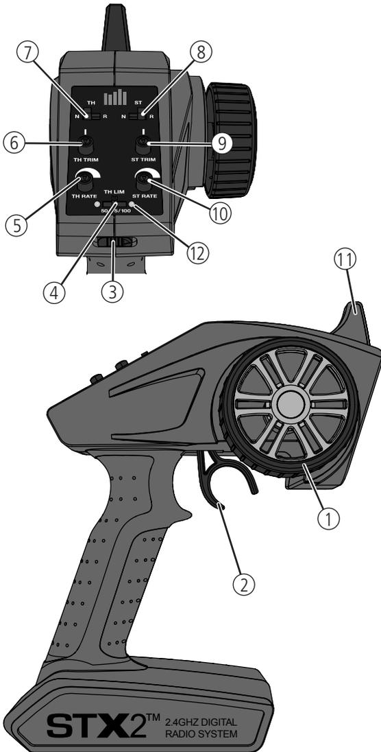
1. **Steering Wheel** Controls direction (left/right) of the model
