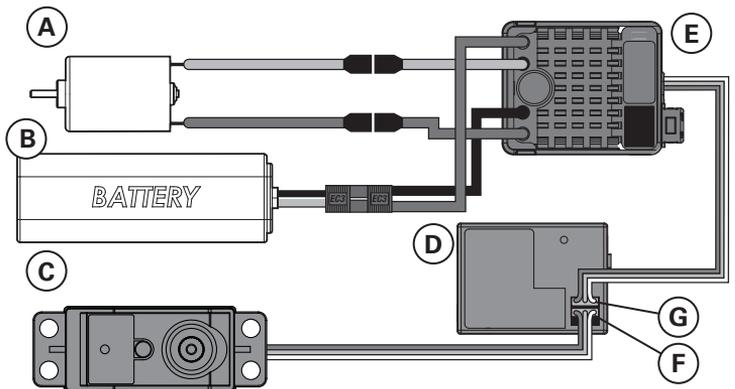
For correct operation, Channels 1 and 2 must be used as shown in the wiring diagram. The motor can be disconnected from the ESC at the connectors in the wiring.
