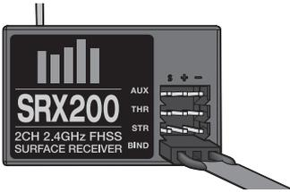
1. With the vehicle on a flat, level surface, insert the Bind Plug in the BIND port on the receiver.
