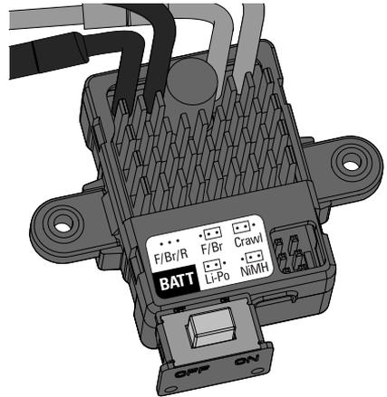
**NOTICE:** Only use the Ni-MH port when using Ni-MH batteries. Using the Ni-MH port with a Li-Po battery can cause serious damage to the battery and is unsafe.
