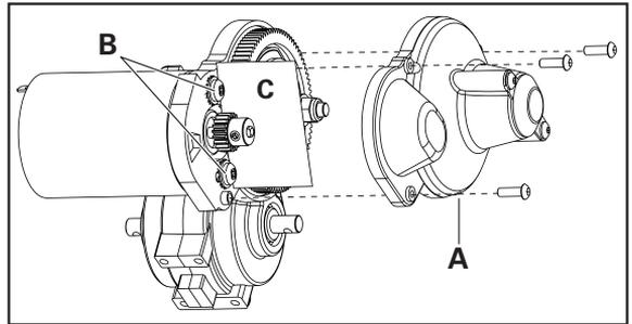
4. Rotate the gears to remove the paper. The gearing should move a small amount.
