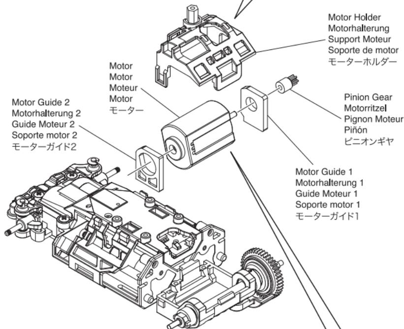
● Remove the Pinion Gear.
