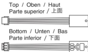
▶ Surface without electric parts (top) faces upwards.
