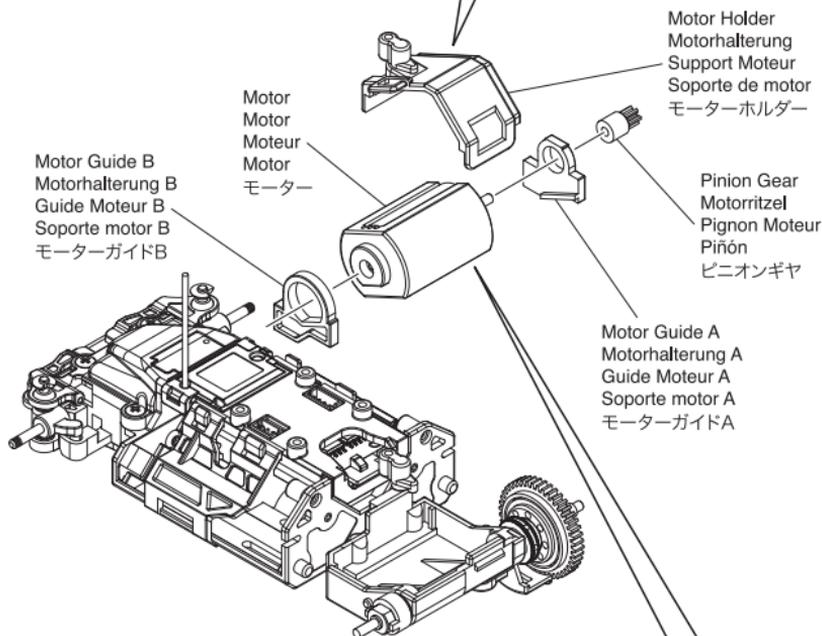
● Remove the Pinion Gear.
