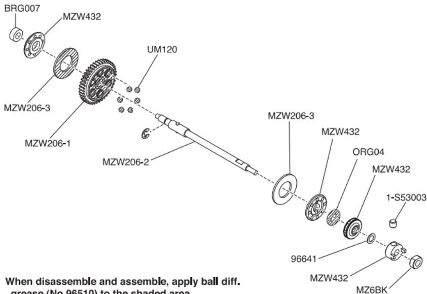
When disassemble and assemble, apply ball diff.
