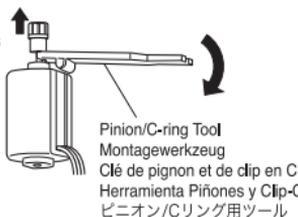
● Install the Pinion Gear.
