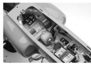
In helicopters, there is generally enough room on the servo tray to achieve the necessary separation. If necessary a mount can be fashioned using clear plastic to mount the external receiver.
