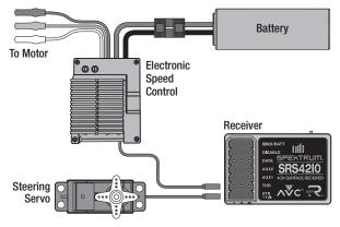
**IMPORTANT:** If you adjust the steering and throttle trim on your transmitter, the receiver must be turned off and back on again in order to save the new trim settings. Otherwise, AVC will not function properly.
