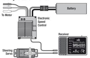
**IMPORTANT:** If you adjust the steering and throttle trim on your transmitter, the receiver must be turned off and back on again in order to save the new trim settings. Otherwise, AVC will not function properly.
