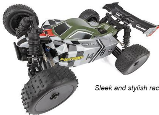
Adjustable turnbuckles and aluminum steering rack
