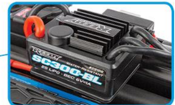
Water-resistant high-power Reedy brushless speed control
