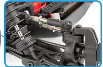
Adjustable turnbuckles and aluminum steering rack
