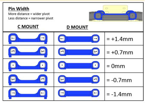
These are some of the possible and most popular toe and anti-squat combinations when using adjustable inserts. The same toe and anti-squat angles can be achieved by using different combinations of inserts but will differ in pin width and height. Take note of these differences when making adjustments.
