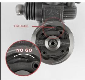
Worn-out clutch shoes can negatively impact the performance of the clutch and cause an engine to intermittently flame out even when tuned properly. This decreases a vehicle's overall performance and can cause headaches at the track.
