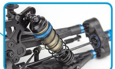
16mm Big Bore 6061 aluminum shock bodies and bleeder-style caps, with new 20mm I.D. springs
