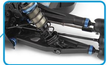
133mm CVA driveshafts increase traction and chassis support
