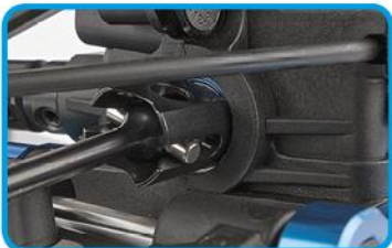
Updated gearbox reduces differential movement for a more consistent gear mesh
