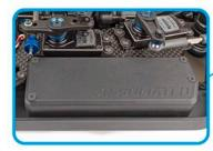
Enclosed battery box for quick and easy battery removal
