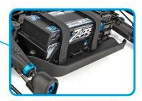
Side guards are now threaded into the chassis from the top side of the car
