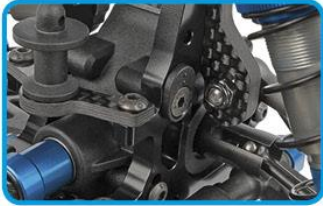
Quick-change adjustable differential height with 7075-T6 aluminum bulkheads
