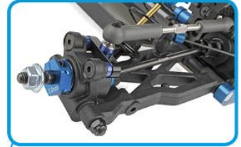
Optimized suspension arm geometry with improved durability and stiffness
